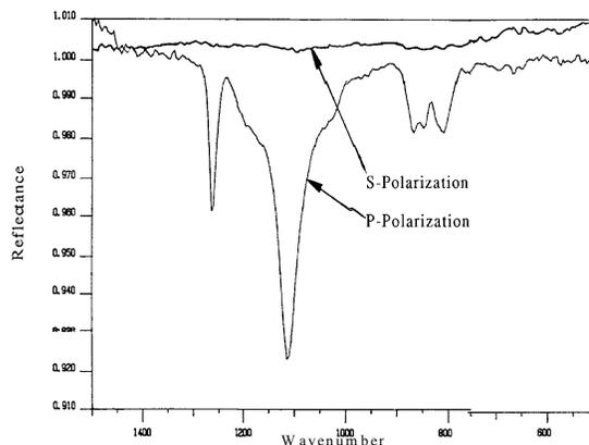
Figure 3. Spectra of Silicone Lubricant on an Al Substrate.
